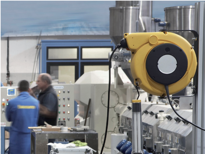
Completely assembled and preset spring-driven cable reel
